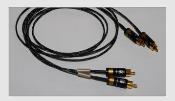
The expirience in winding finest internal wirings of purest copper for our tonearms made us following this philosophy for phono-, line- and speaker-cables. They are available in different length with free choice for input and output-plugs. Each conductor is made of several ultra-thin copper wires, pairwise twisted and casted into nylon. The cable is mechanically flexible to keep away airborne vibrations from the gear.
