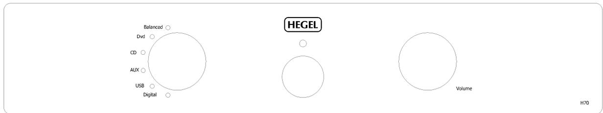
The amplifier is switched on with the button in the middle of the front panel. A blue light indicates it is switched on.
