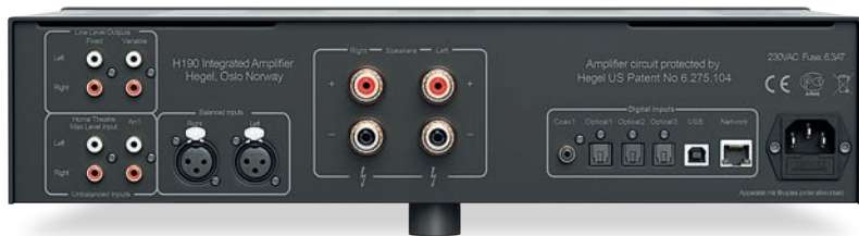
ABOVE: To the left of the rear panel are fixed and variable level preamp outs, plus two sets of RCA ins and one balanced XLR pair. The digital section has three optical and one coaxial in, a USB Type B and an Ethernet port for computer connection
